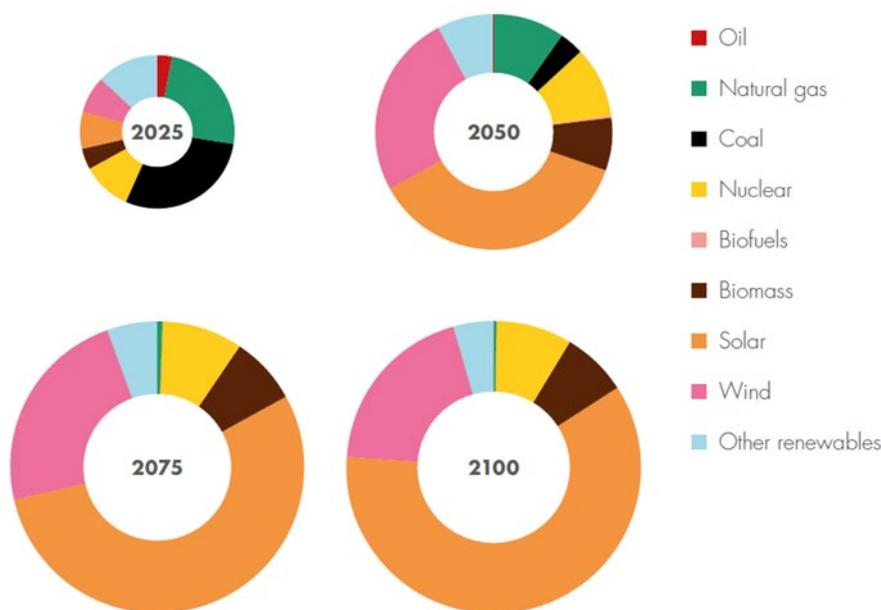
**Figure 49: Development of global power generation by technologies in the Sky-Scenario; the diameter of the pie charts corresponds to the global power requirement [Shell]**
