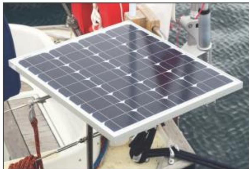
*An adjustable stem rail mount holds a conventional rigid solar panel (fingers and busbars on the top of the panel). Again, these are half cells to boost the voltage to battery-charging levels in a relatively small panel.*
