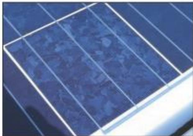
The bluish color and multiple alignments of the crystals in this rigid panel clearly indicate that these are polycrystalline, or multicrystalline, cells.
