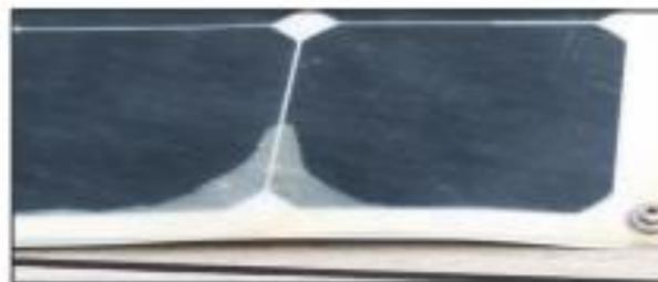
*Delamination of a semi-flexible solar panel is a common failure. Once again, these are SunPower Maxeon cells.*
