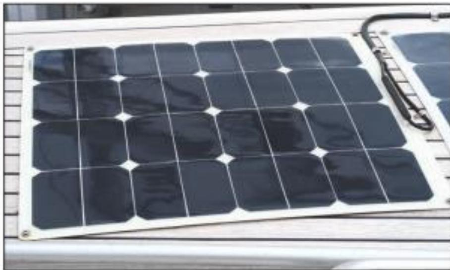
The uniform black indicates that these are monocrystalline cells, while the lack of any fingers or busbars tells us they are SunPower's Maxeon cells, in this case, mounted in a semi-flexible panel.
