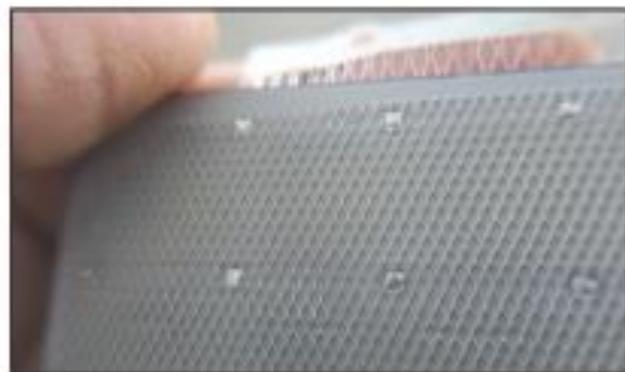
A Merlin MTAT energy-collection grid for the back side of a solar cell—with many connection points and short energy paths to the grid—lowers resistance, increases efficiency, and can significantly minimize the effects of any cell cracking and other damage.
