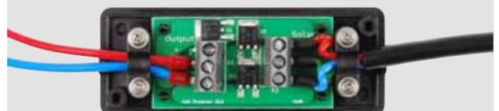
With this hookup, the cells are protected with 2 bypass diodes against the hot spot effect and the additional blocking diode protects against reverse current back into the module. By damage to a module or cable by several modules in parallel operation, an influence can be prevented on the other modules with the use of the blocking diode.
