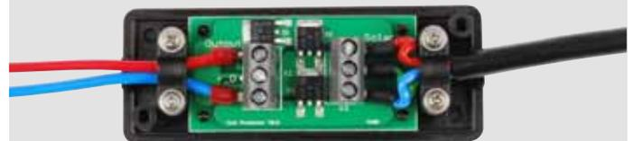
With this hookup, the cells are protected with 2 bypass diodes against the hot spot effect.
